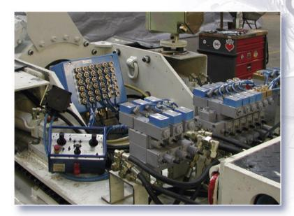
Intrinsically safe valve solenoids iEA33 on a hydraulic control block for the operation of an electrohydraulically driven drilling carriage underground
