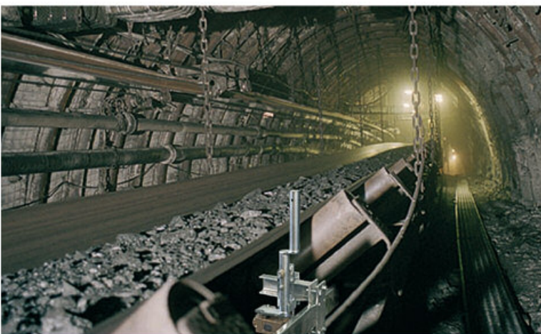
Magnet switch iKA209 for conveyor belt monitoring
