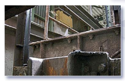
Magnet switch iKA509 used for hoisting cage position monitoring
