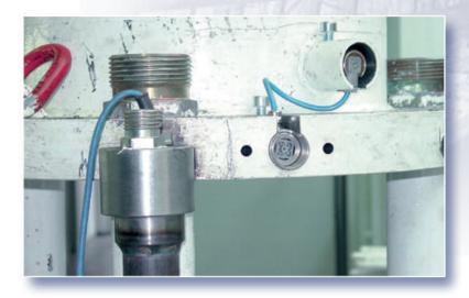
Monitoring the closing action at the pipe piston conveyor
